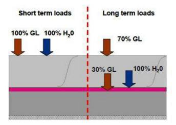
Figure 14: Load sharing between primary and secondary SCL linings [10]
