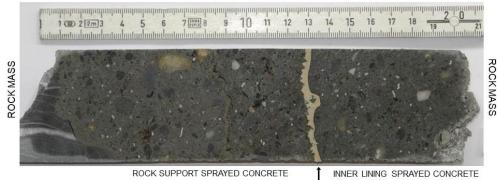
DOUBLE BONDED SPRAY-APPLIED WATERPROOFING MEMBRANE Figure 12: Drill core sample from the complete final waterproof lining [8], drill location shown
