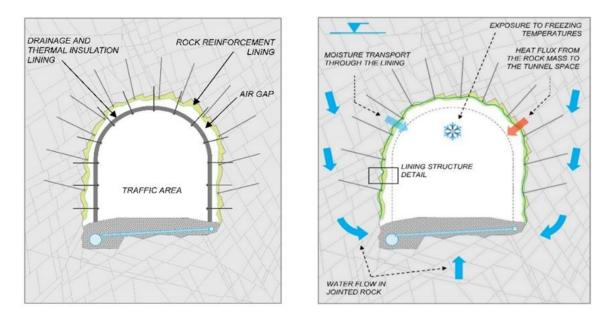
Figure 11: Cross sections of the final inner lining of the Gevingås rail tunnel. Left: Original design with the PE foam sheet drainage system, realized in 2200 m of the tunnel length. Right: the alternative and innovative design with sprayed concrete and spray-applied water-proofing in the final inner lining, realized in 1850 m of the tunnel length. The waterproof redirects the water flow as shown [7]
