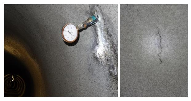
Figure 8: Manometer indicating 4 bar water pressure [Master Builders Solutions]
