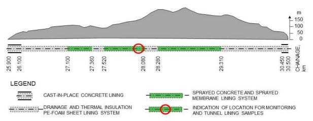
Figure 10: Longitudinal section of the Gevingås rail tunnel, total length 4100 m, showing the different constructed lining types [6]
