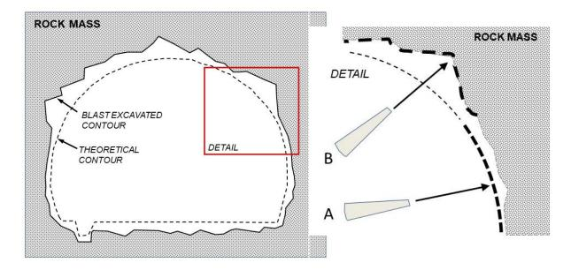
Figure 11: Application of sprayed concrete on a blast excavated rock surface. Detail A indicates ideal spray angle and nozzle distance with an even rock surface. Detail B illustrates the importance of the nozzle following the uneven rock surface in order to avoid severe inhomogeneities and poor compaction
