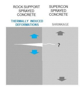
Figure 8: Loading model for the deformation exposure at cracks in the rock support sprayed concrete lining
