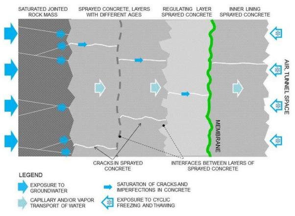
Figure 6: Cross section with details and waterproofing function for a tunnel lining with sprayed concrete in combination with a spray-applied membrane [1]
