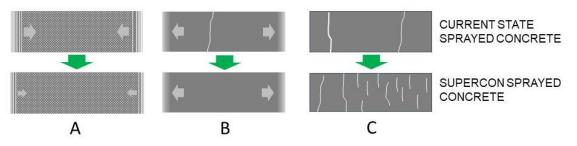
Figure 10: Three important sub-targets of material technology development for the SUPERCON project. A: significant reduction of shrinkage. B: significant increase in ductility represented failure strain in uniaxial tension. C: significant distribution of cracks in concrete with the use of fibre technology
