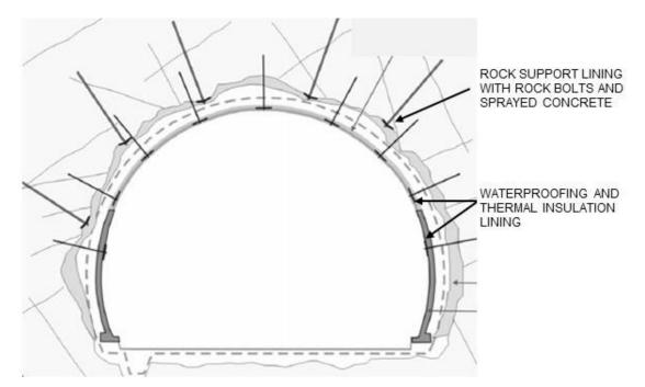
Figure 1: Principal layout of the lining design for traffic tunnels in Norway, with the two functional parts: the rock support lining and the water and frost protection lining. Modified after Broch et al [3]
