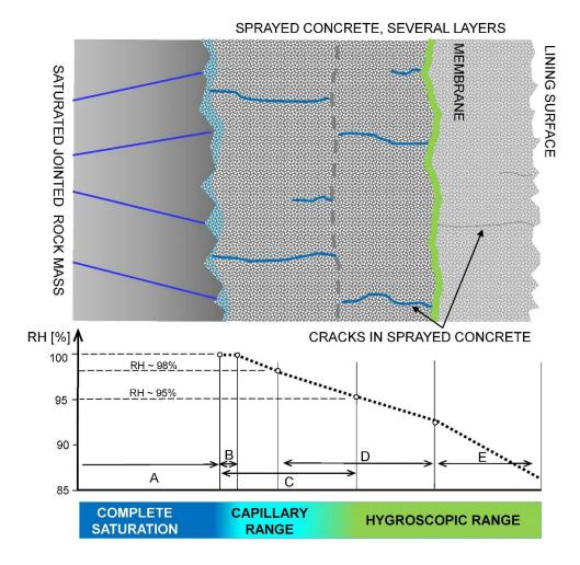
Figure 9: Principal model for moisture condition in an undrained and bonded lining structure given as relative humidity (RH) and moisture transport mechanisms [5].
