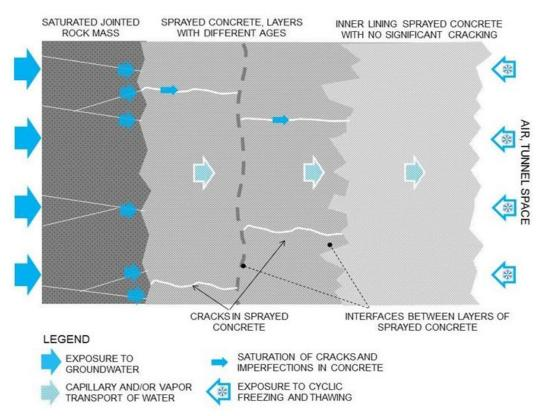
Figure 7: Cross section of lining details with the main intended area of use for the sprayed concrete technology in the SUPERCON project: a functional waterproof layer based on sprayed concrete to be applied onto the rock support lining
